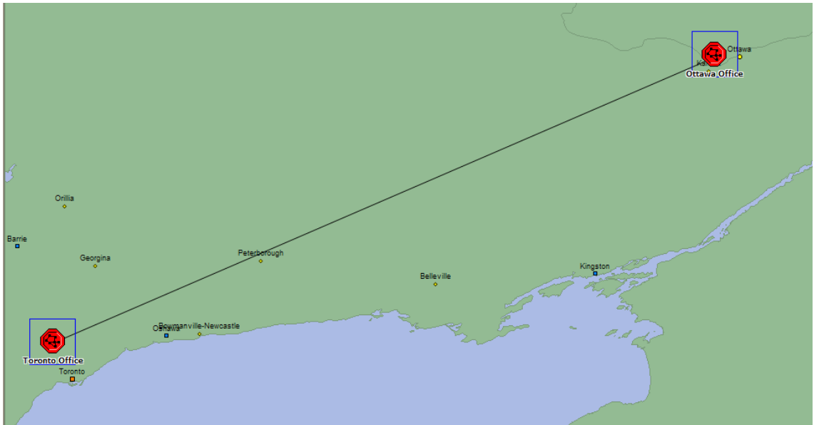
Figure 4.14 Network topology. Toronto office and Ottawa office interconnected by a DS1 link.
